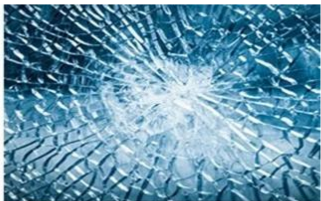
Tempered glass breaks into many small pieces with less sharp edges.
