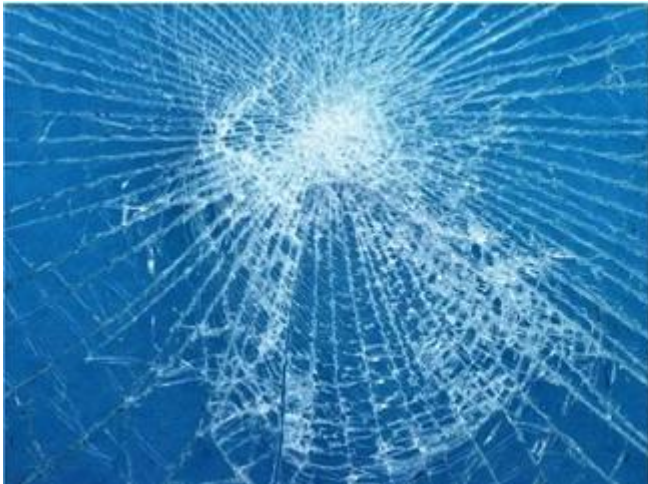
Non- tempered laminated glass broken
