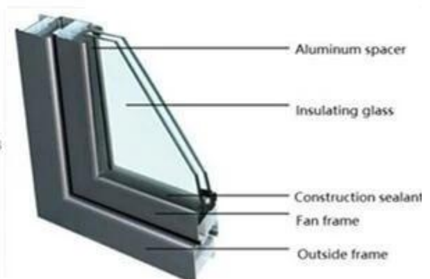
Aluminum spacer insulated glass
